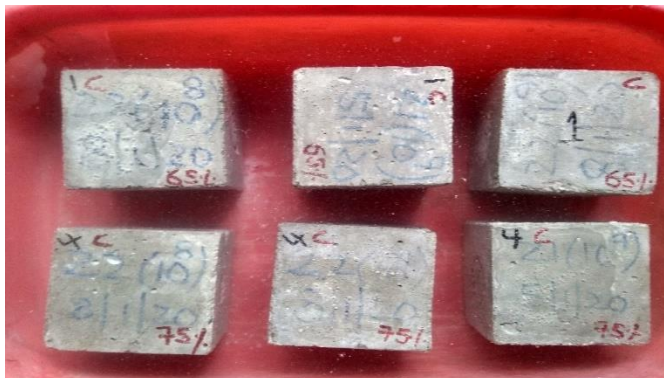
Fig. 2 Experimental setup for water absorption test
