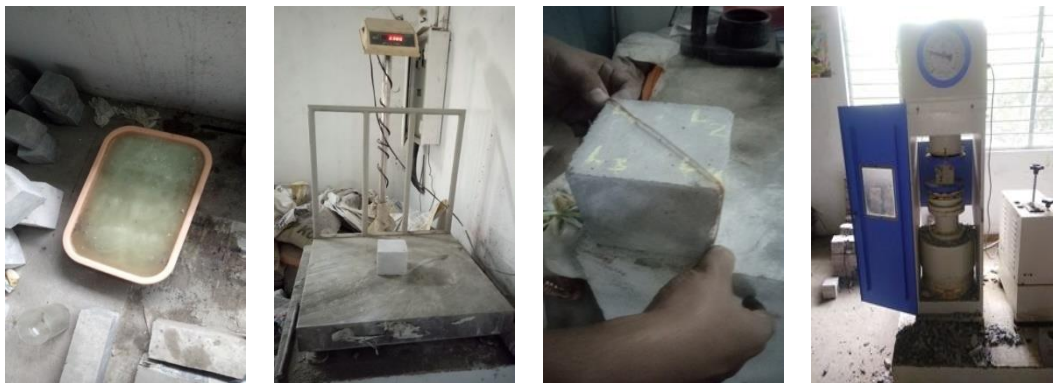
Fig. 3 Experimental setup for acid attack test
