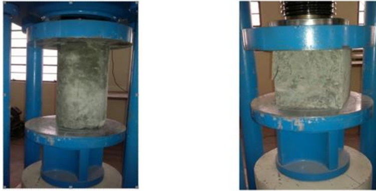
Fig. 1. Compressive strength test arrangement for Cylinder and cube
