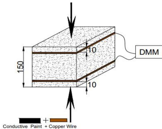
Fig. 2. Specimen details for stress sensing test
