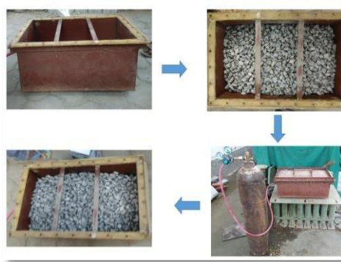
Fig. 4 Carbonation treatment to RFA
