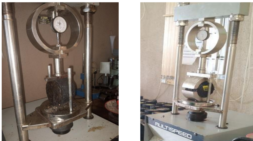
Fig. 3 Specimen under (a) ITS test (b) Marshall Stability test.
