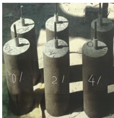
b) Cast cylinders with rebar
