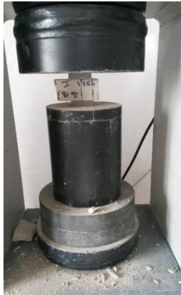
Fig. 8 Compressive test showing the crushing of specimen.
