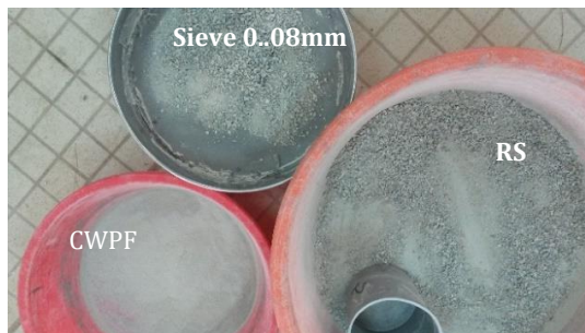
Fig. 5 Preparation of fines by sieving
