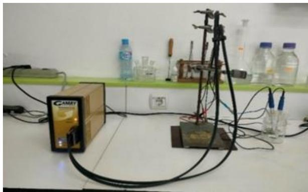
Fig. 3. Corrosion test Gamry 600+ cell [29]
