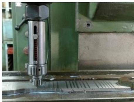
Fig. 2. Setup photo of the burnishing operation[29]
