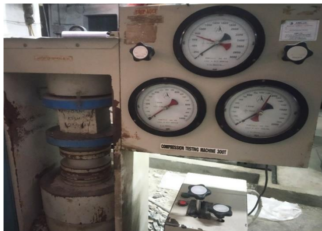
Fig. 4. Compressive strength test using 300T CTM
