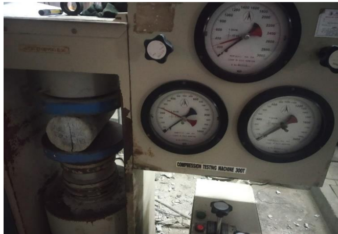
Fig. 6. Split tensile strength test using 300T CTM
