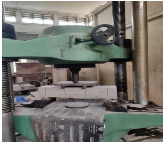
Fig. 8. Flexural strength test using 100T UTM
