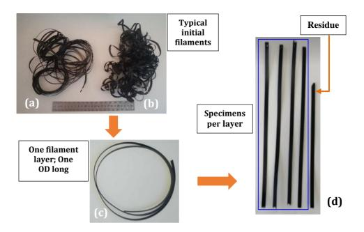
Fig. 7. Steps for testing specimen cutting
