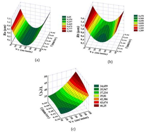
Fig. 5. Estimated response surface of performance characteristics versus Vc and f
