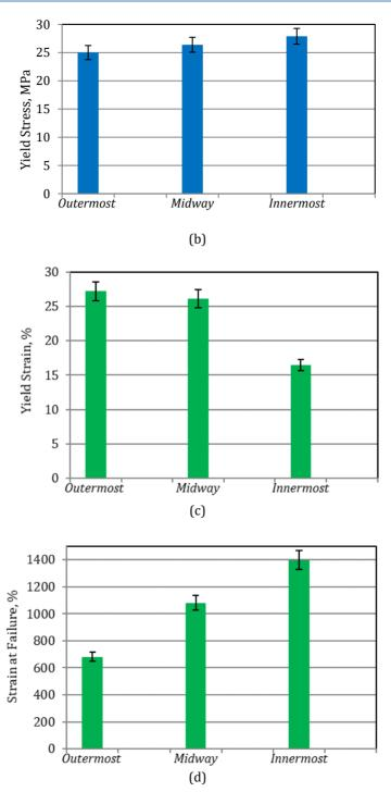
Fig. 10. Evolution of (a) E, (b)  $\sigma_{y}$ , (c)  $\epsilon_{y}$  and (d)  $\epsilon_{f}$  as a function in pipe wall
