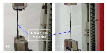
Fig. 8. Photographs of filament behavior under monotonic traction
