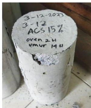
Fig. 7. Sample concrete after compression test
