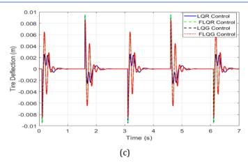
Fig. 10. Comparison of closed-loop responses (Case 1)
