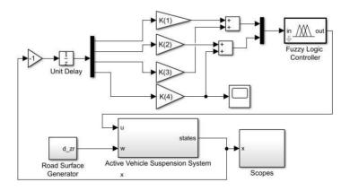
Fig. 2. FLQR control structure
