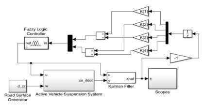
Fig. 9. FLQG control structure of the active vehicle suspension system
