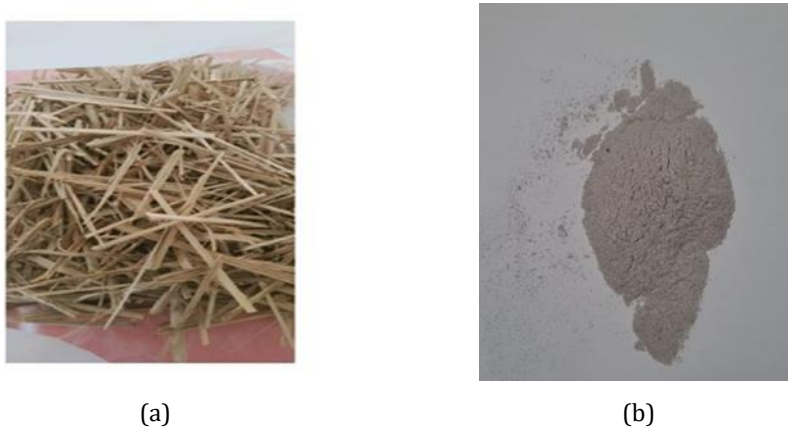
Fig. 2. (a) Rattan fiber, (b) clam shell ash
