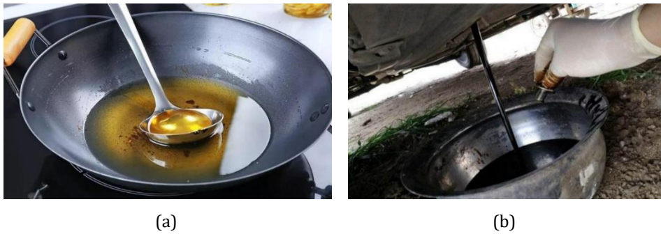
Fig. 2. Rejuvenators used in the study (a) discarded waste cooking oil (WCO) and (b) waste engine oil (weo) collected from automobile workshop
