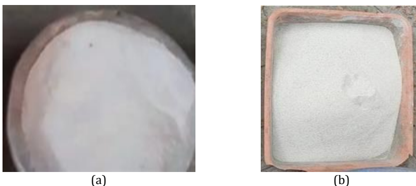
Fig. 1. (a) Calcium carbonate powder and (b) calcium carbonate sand
