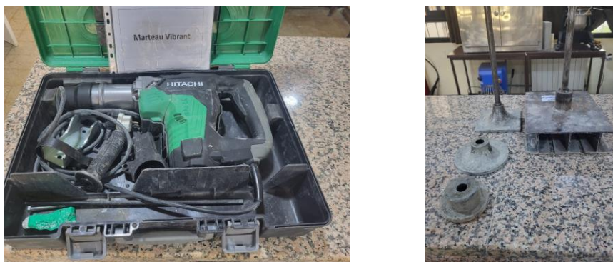
Fig. 6. The vibrating hammer employed for compacting the RCC specimens
