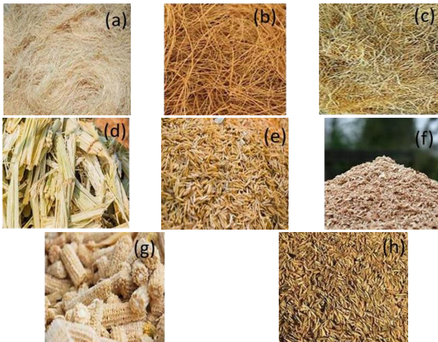
Fig. 1. Agro-waste utilized for particleboard manufacture (a) Areca nut fiber, (b) Coconut fiber, (c) Rye straw, (d) Sugarcane bagasse, (e) Rice husk, (f) Sawdust, (g) Corncob, (h) Oat hulls
