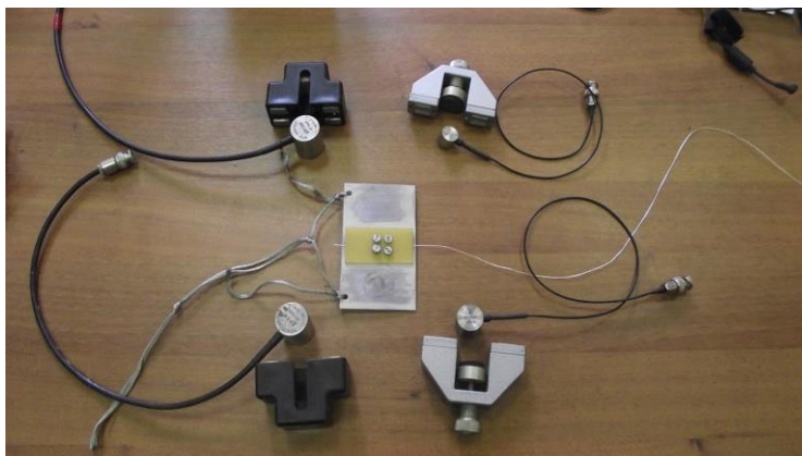
Fig. 2. AEC is used in conjunction with a waveguide grip
