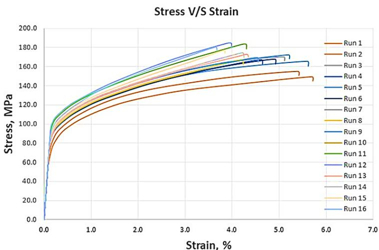
Fig. 4. Stress-strain curve of the produced composites at different runs
