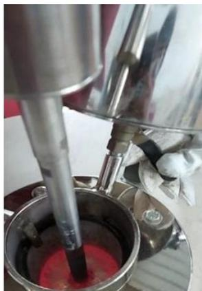
Fig. 2. Stirring of molten metal
