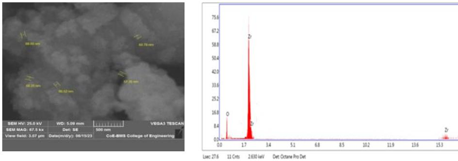
Fig. 12. EDS Spectrum of n-ZrO<sub>2</sub>
