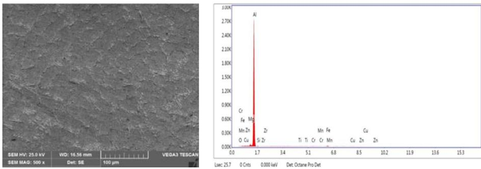
Fig. 13. EDS Spectrum of Al6061/1%ZrO<sub>2</sub>/1%Al<sub>2</sub>O<sub>3</sub>
