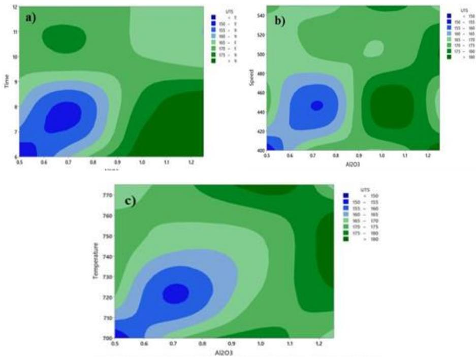
Fig. 9. Contour plots of UTS with various process parameters with respect to wt% of Al<sub>2</sub>O<sub>3</sub>
