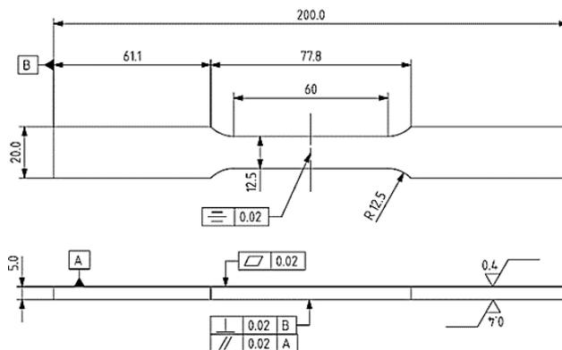
Fig. 3. Tensile specimen specification
