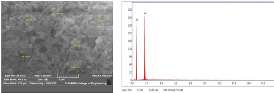
Fig. 11. SEM and EDS Spectrum of n-Al<sub>2</sub>O<sub>3</sub>
