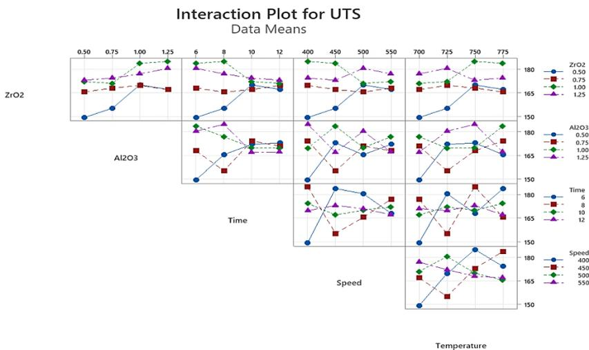
Fig. 7. Interaction plot for UTS of Al6061/ZrO<sub>2</sub>/Al<sub>2</sub>O<sub>3</sub>
