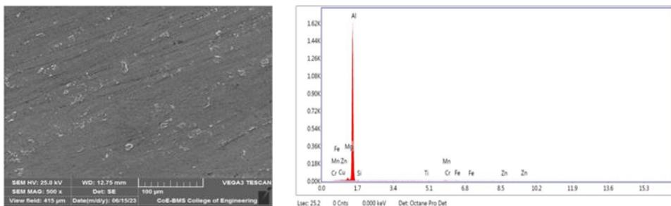
Fig. 10. SEM and EDS Spectrum of Al6061
