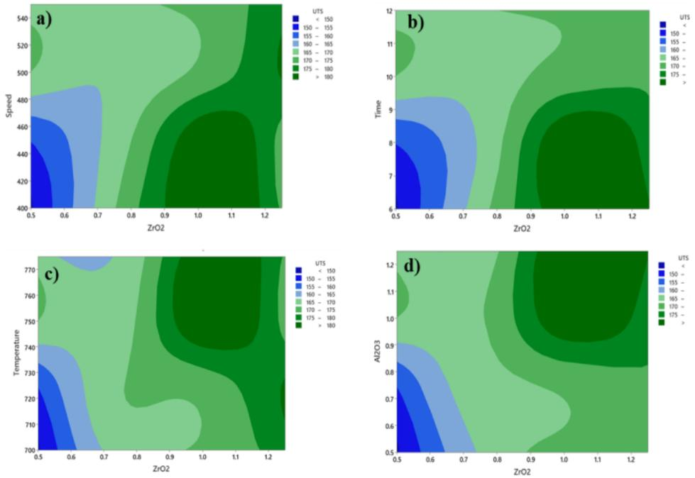
Fig. 8. Contour plots of UTS for various process parameters with respect to wt% of ZrO<sub>2</sub>
