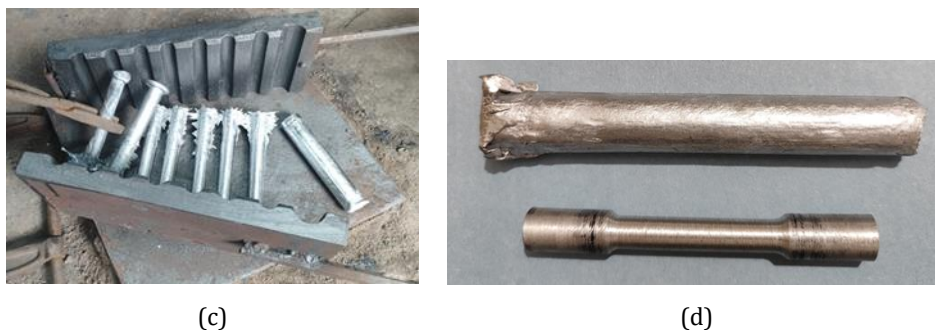
Fig. 2. Showing the (a) Furnace set up (b) Cast iron die (c) Casting in die (d) Sample of casting and tensile test specimen
