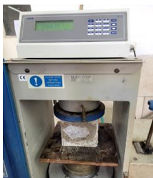
Fig. 17. Testing the Failure of a Cubic Specimen Using a Concrete Breaker Jack
