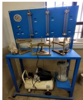
Fig. 12. Concrete Permeability Device and Its Test Results
