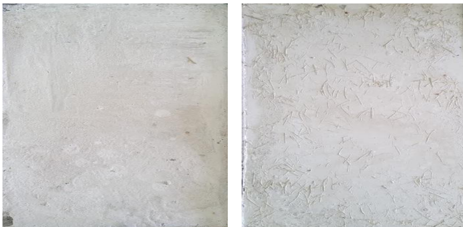
Fig 15. Concrete slab reinforced with fibers
