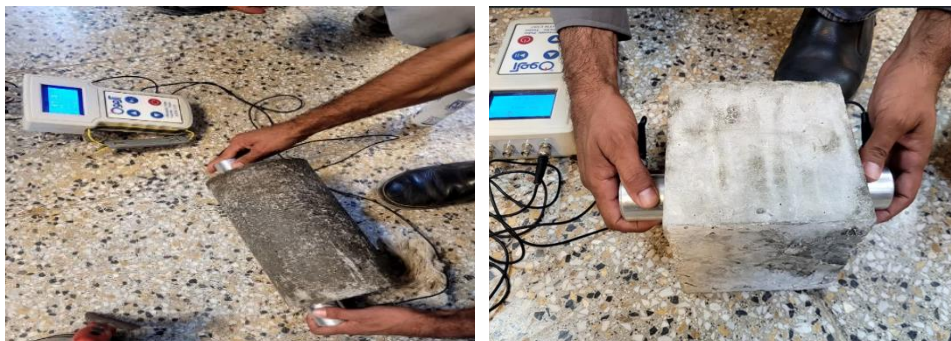
Fig. 10. UPV Testing on Cubic and Cylindrical Specimens
