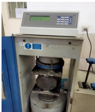
Fig. 19. Cylindrical Specimen Failure Test Using a Concrete Breaker Jack
