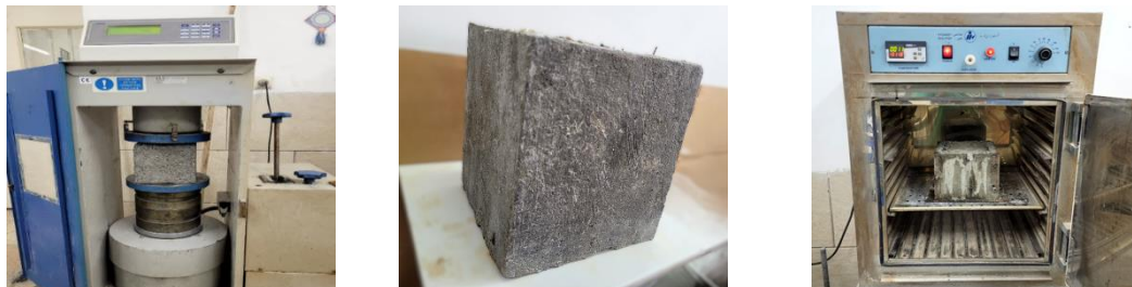
Fig. 13. Cube testing in the drying oven and failure using the compressive strength device.
