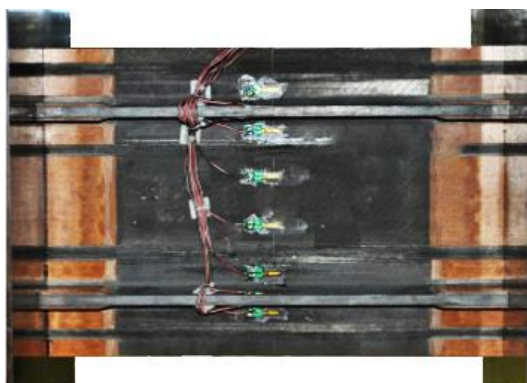
Fig. 1. Double-stringer panel on the test bench before fracture
