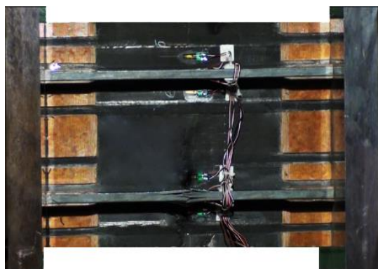
Fig. 2. Double-stringer panel on the test bench after fracture
