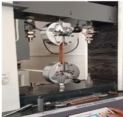
Fig. 6. UTM with Tensile Sample Loaded
