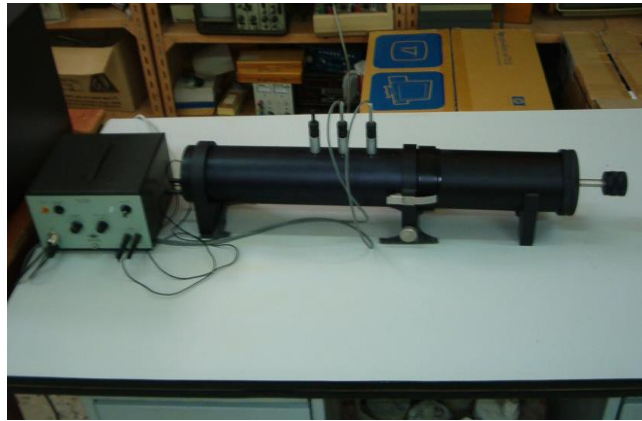
Fig. 2. Equipment used to measure \alpha (Double Microphone System Model 4206)
