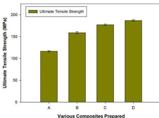
Fig. 6. Ultimate tensile strength of A356 alloy with nano graphene and SiO<sub>2</sub> particles reinforced composites
