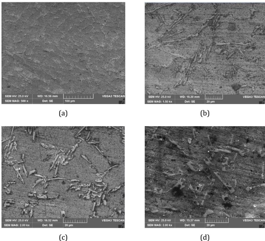
Fig. 4. SEM Micrographs of (a) As-cast A356 alloy (b) A356-1 wt.% of Gr and 2.5 wt.% of  $\text{SiO}_2$  Composites (c) A356-1 wt.% of Gr and 5 wt.% of  $\text{SiO}_2$  Composites (d) A356-1 wt.% of Gr and 7.5 wt.% of  $\text{SiO}_2$  Composites
