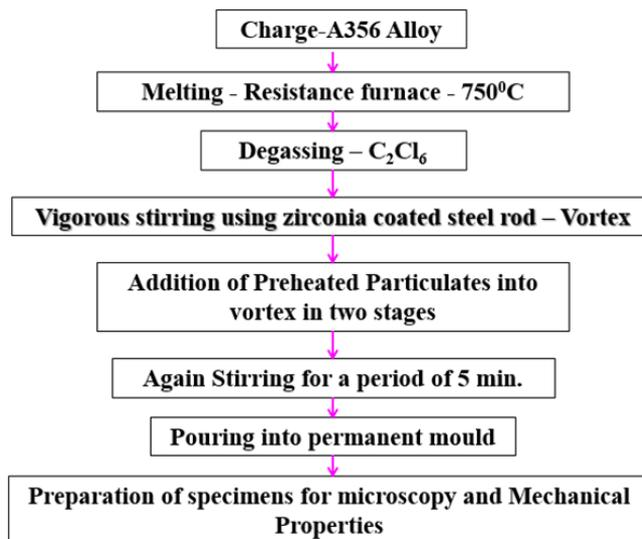
Fig. 1. Process of preparing A356 alloy hybrid composites
