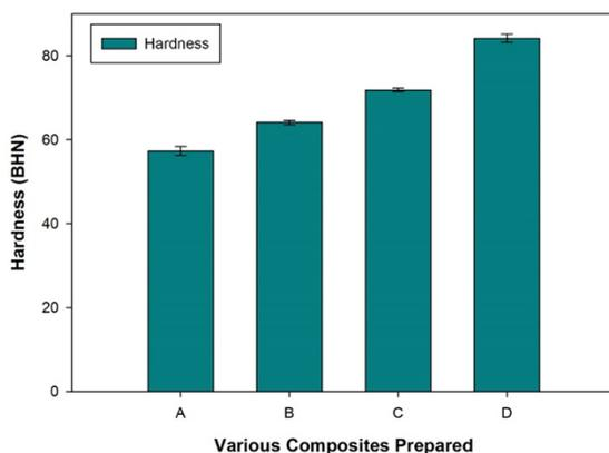
Fig. 10. Hardness of A356 alloy with nano graphene and SiO<sub>2</sub> particles reinforced composites
