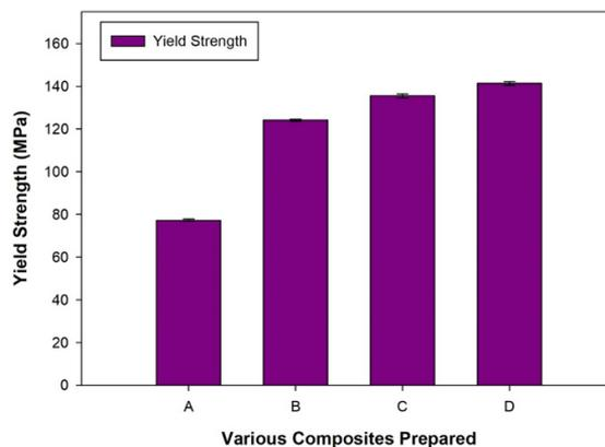
Fig. 7. Yield strength of A356 alloy with nano graphene and SiO<sub>2</sub> particles reinforced composites
