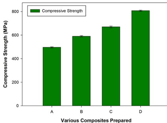
Fig. 9. Compressive strength of A356 alloy with nano graphene and SiO<sub>2</sub> particles reinforced composites
