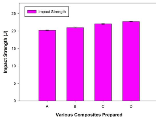
Fig. 11. Impact strength of A356 alloy with nano graphene and SiO<sub>2</sub> particles reinforced composites
