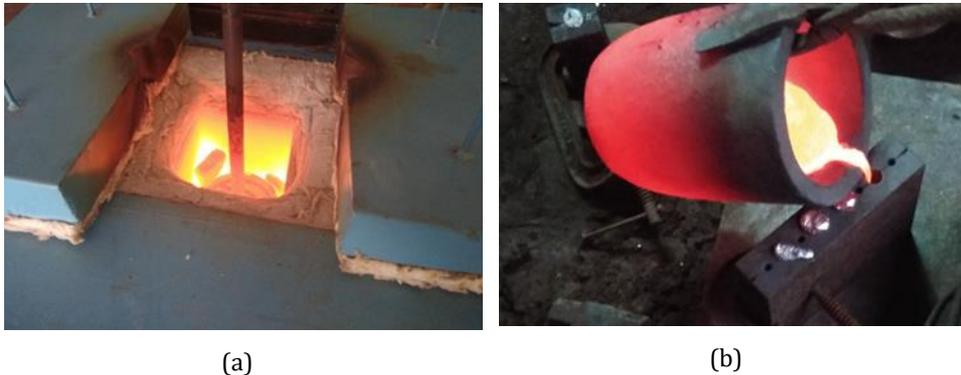
Fig. 2. Showing the (a) Molten metal in electric furnace (b) Cast iron die used to prepare samples
