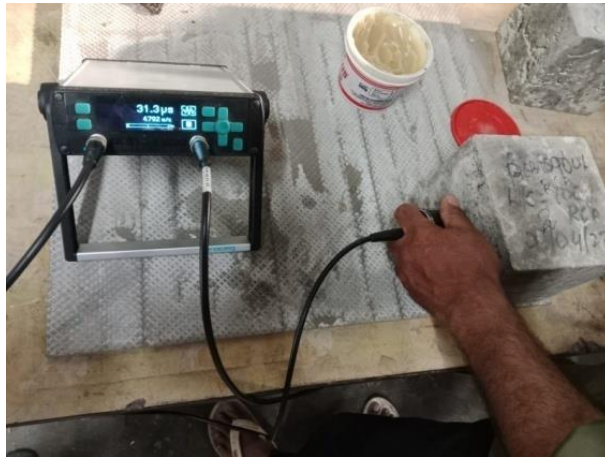
Fig. 13. Ultrasonic pulse velocity test
