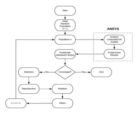
Fig. 2 Flowchart of the implemented Genetic Algorithm.
