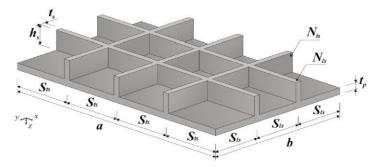
Fig. 1 Stiffened plate with 2 longitudinal and 3 transverse stiffeners
