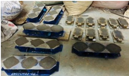
(c) Cement-sludge mortar preparation
