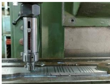
Fig. 2. Setup photo of the burnishing operation[29]
