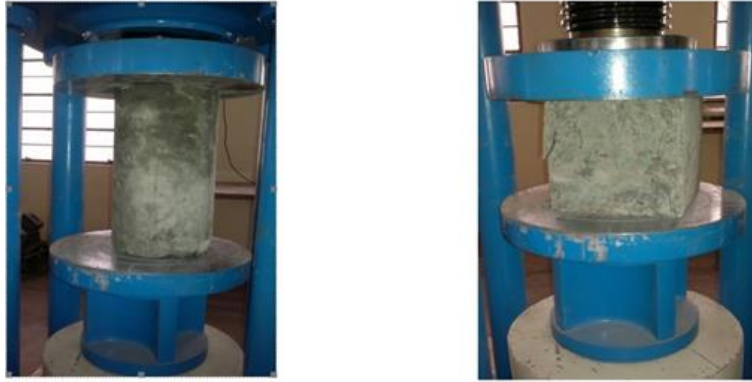
Fig. 1. Compressive strength test arrangement for Cylinder and cube
