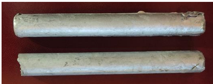
Fig. 5. Al7085 alloy -B 4 C composites after casting
