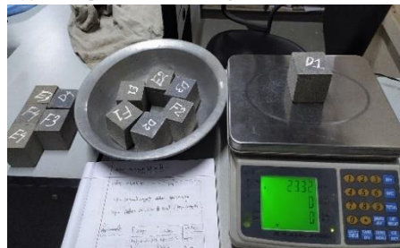
(h) Water absorption test
