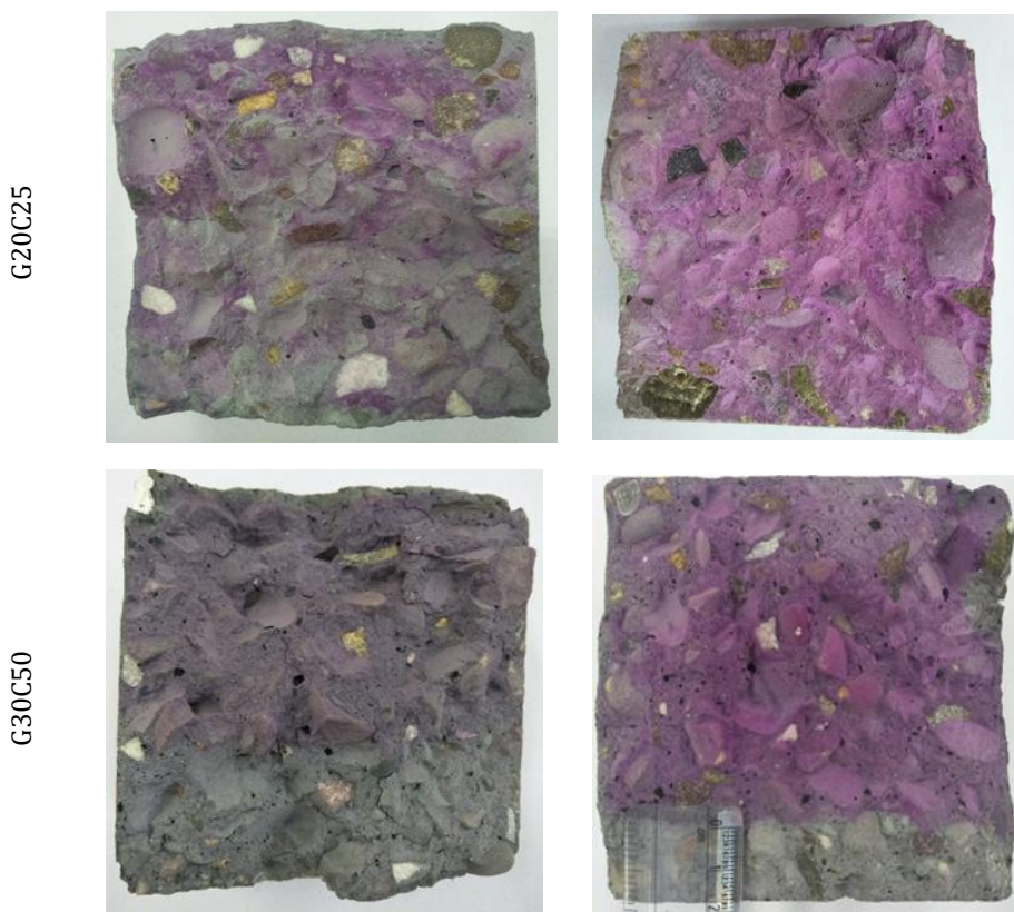
Fig. 6. Carbonation depth as observed in various specimen of different concrete mix after 28 day-4-week carbonation and 90 day-4-week carbonation
