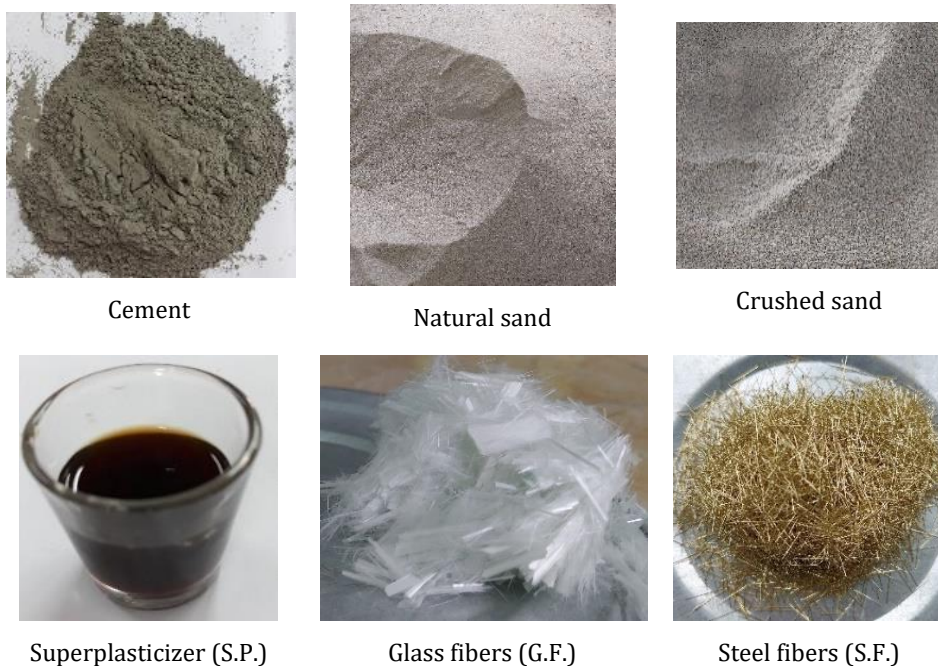
Fig. 3. Materials used for mixing concrete
