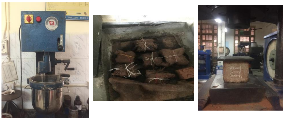
Fig. 3. (a) Mortar mixer, (b) curing of Lime mortar cube, and (c) UTM for compression test
