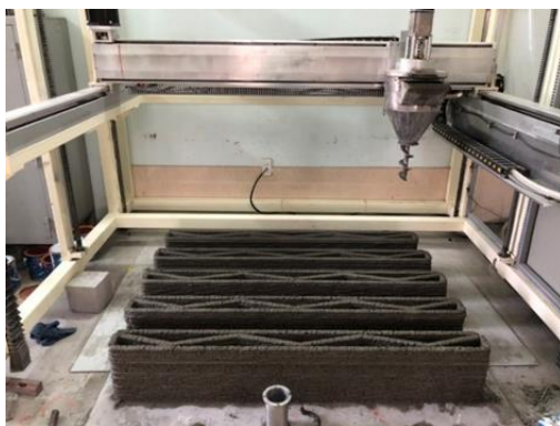
a) WB00 and Glass Fiber beams (GB01 to GB04) (from inside to outside)
