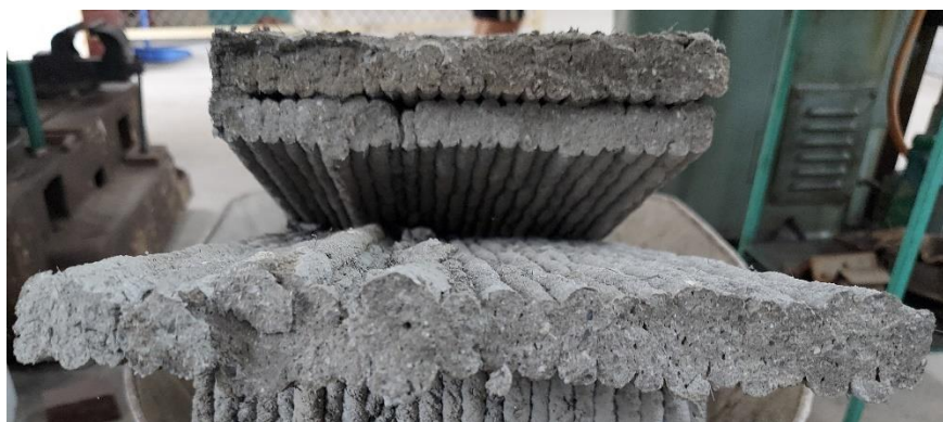
Fig. 13. The surface fracture of the printed beams
