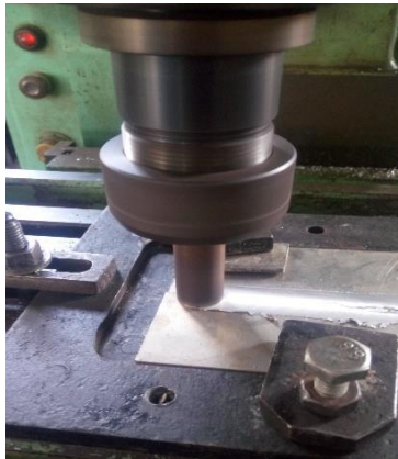
Fig. 1. A non-consumable HSS rotating tool mounted on a vertical milling machine for FSW
