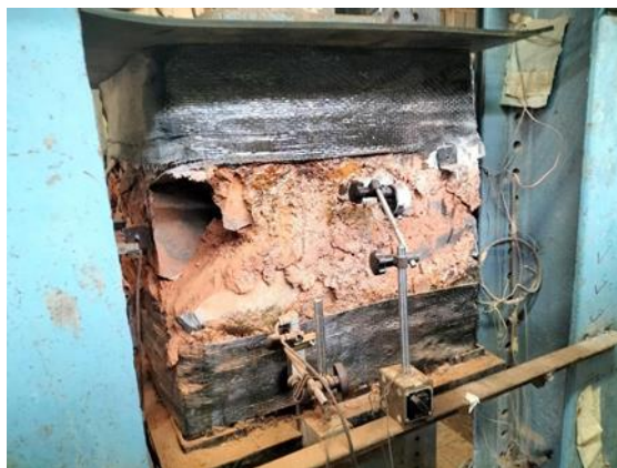
Fig 8 Failure of cube
