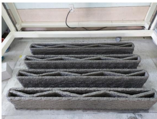
b) Steel Fiber beams (SB01 to SB04) (from inside to outside)
