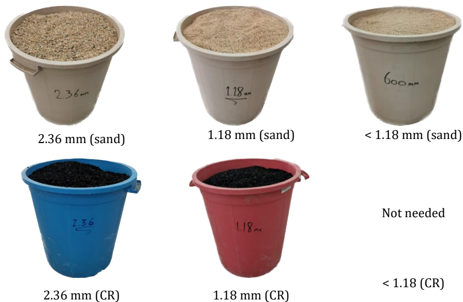
Fig. 3. The classification of particle sizes for sand and CR.
