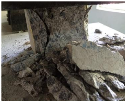
Fig. 1. Failure of cube specimen under compressive load
