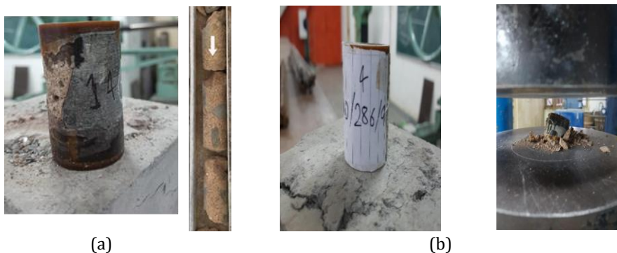
Fig. 2. (a)Core samples before and after capping, (b)Testing of core in CTM
