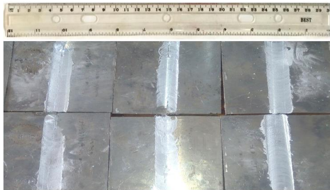
Fig. 5. Some selected reinforced and unreinforced AA6061-T651 friction stir weldments
