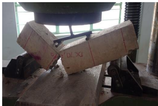
Fig. 3. Flexural test on SCC specimen
