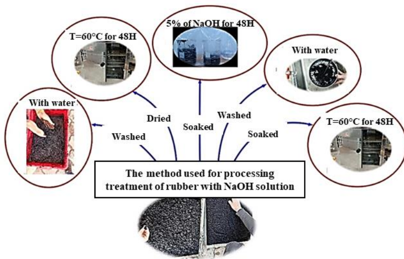
Fig. 5. The method used for processing treatment of rubber particles
