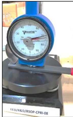
Fig. 4. Hardness testing test rig
