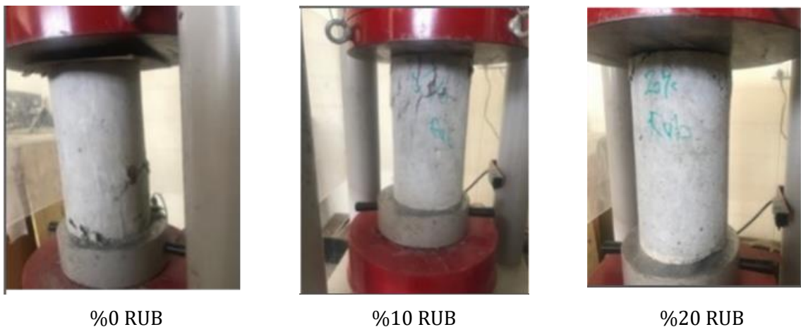
Fig. 5. Failure mechanisms of concrete cylinders following a test for compressive strength
