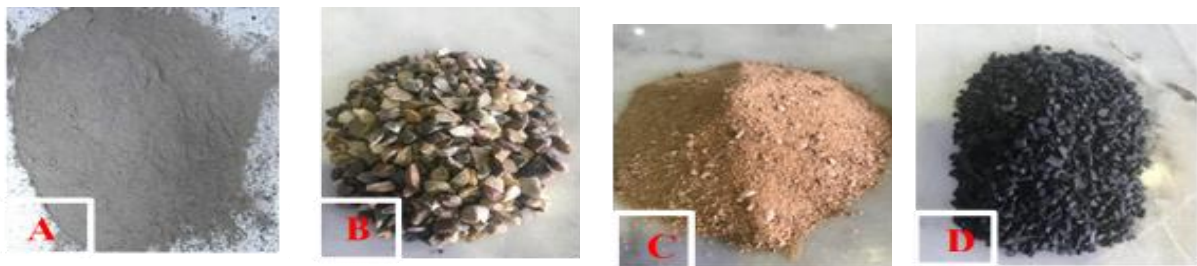
Fig. 1. (A) OPC, (B) crushed coarse aggregate, (C) sand, and (D) rubber aggregate
