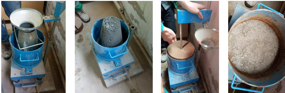
Fig. 7. Vebe test Apparatus for evaluating consistency of fresh RCC
