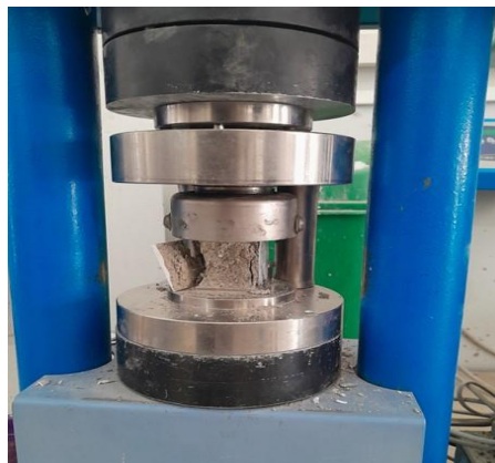
Fig. 5. Compressive strength test of geopolymer mortar
