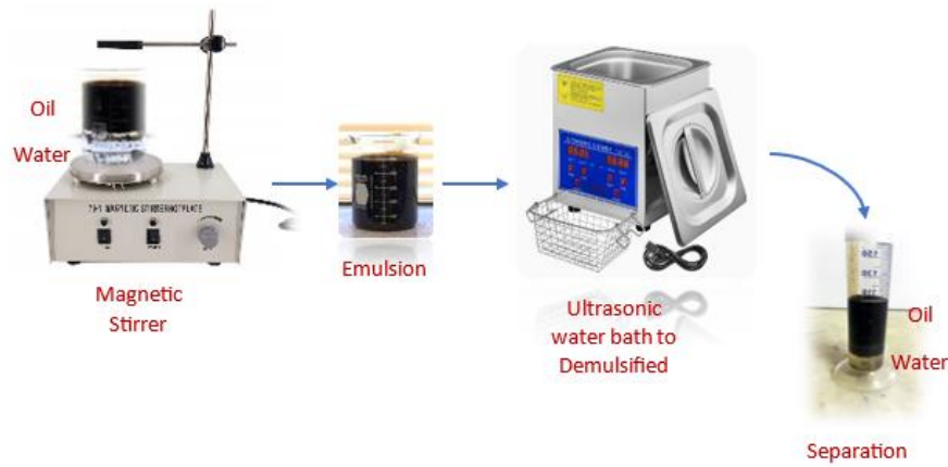
Fig. 2. Separation process water/Oil
