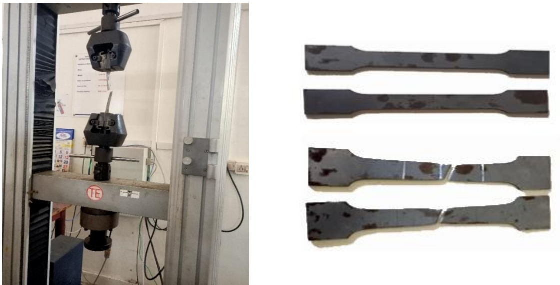
Fig. 2. Tensile test on CFS Coupon specimen
