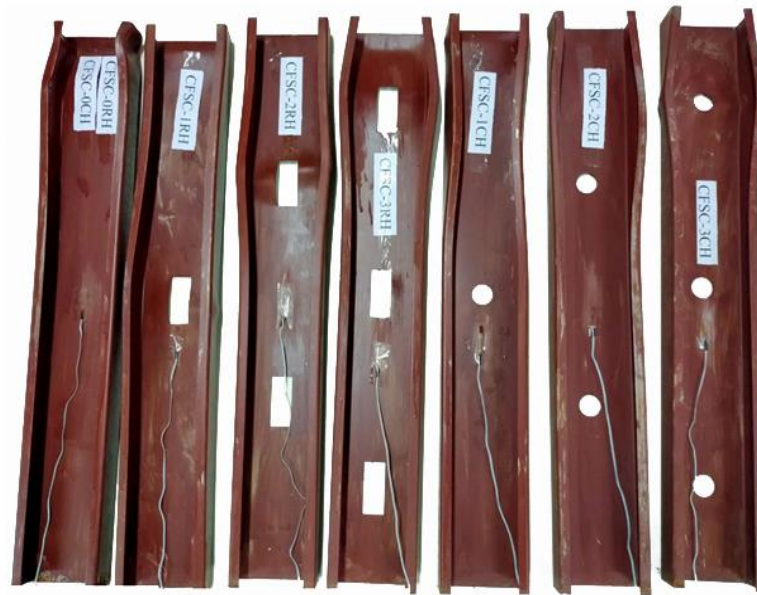
Fig. 10. Failure of the perforated CFS columns
