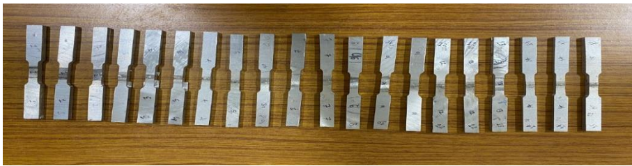
Fig. 4. Photographic representation of tensile specimens
