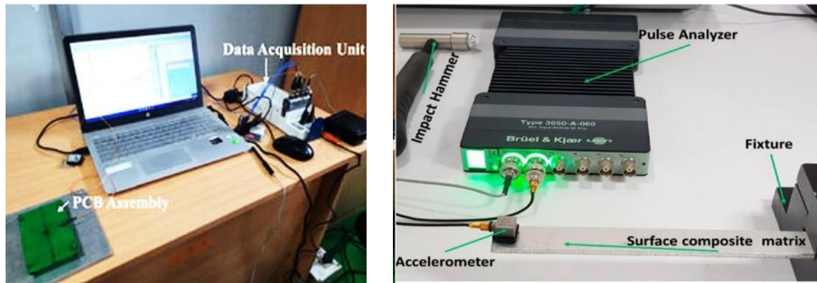
Fig. 3. Free impact vibration 3050 Pulse analyzer
