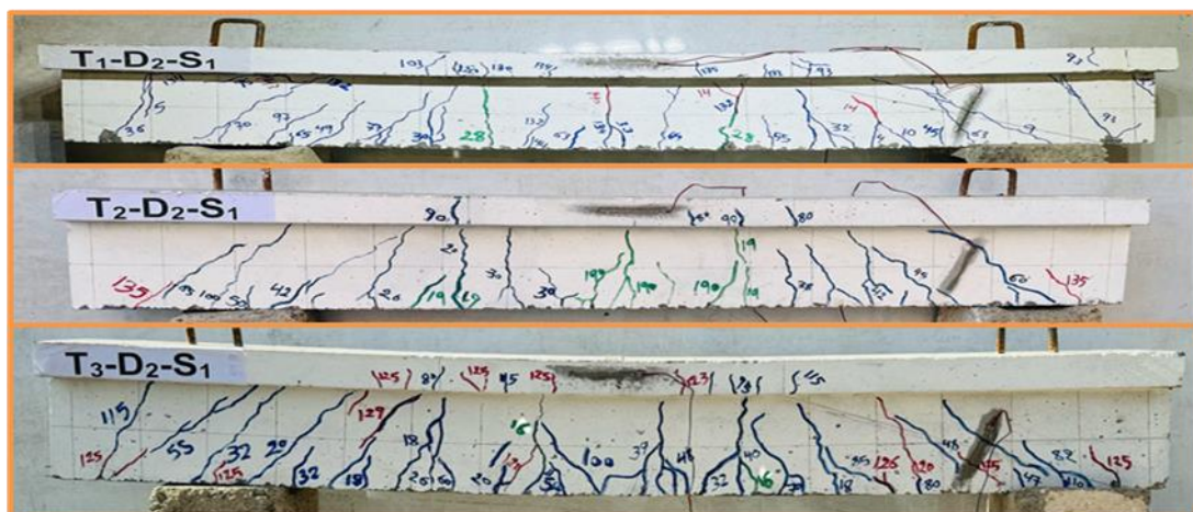
Fig. 12. Crack patterns and failure modes for T-beams reinforced with steel bar of 12 mm
