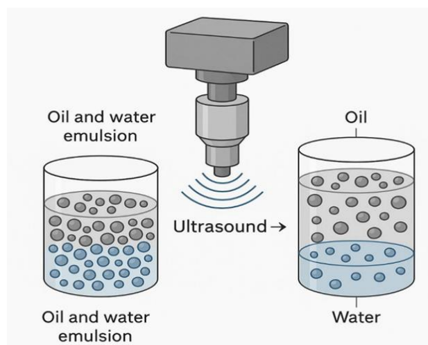
Fig. 1. Mechanism of ultrasonic activity in emulsion separation [11]
