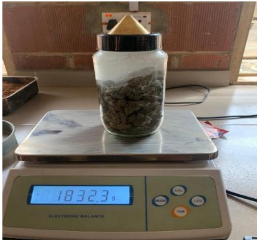
Fig. 3. Particle Density Apparatus – Pycnometer Technique
