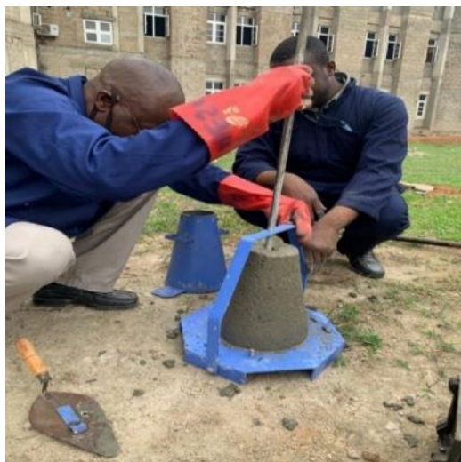
Fig. 7. Experiment on the workability of concrete specimen
