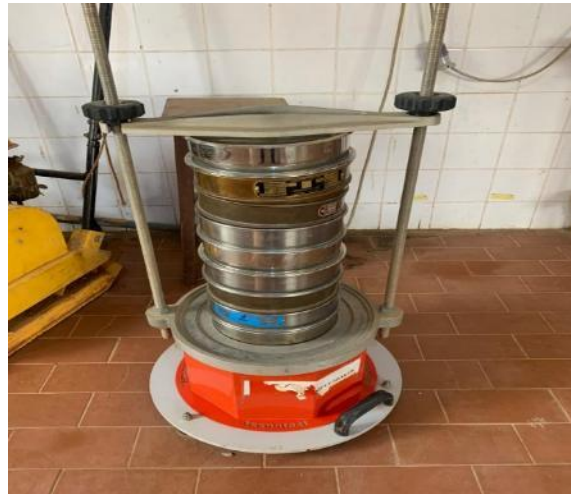
Fig. 4. Set of sieves on sieve shaker
