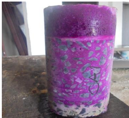
Fig. 10. Carbonation for Phase 1 Mix (0% RAC-Control-CA1) concrete sample
