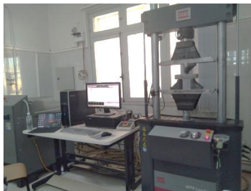
Fig. 8. The ASTM C192 testing set-up
