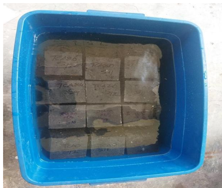
Fig. 12. Sulphate Resistance Test
