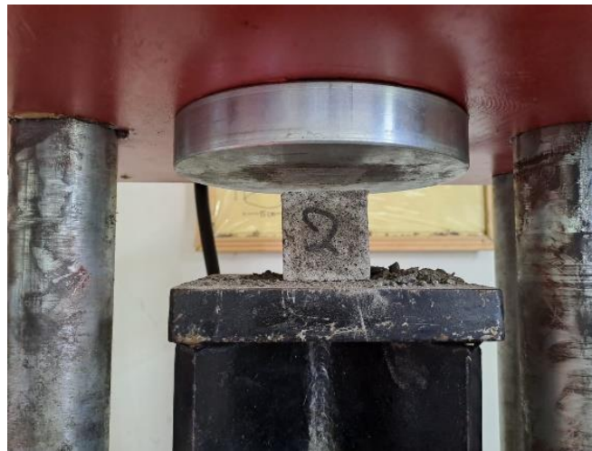
Fig. 3. Compressive strength testing [34,46,47]
