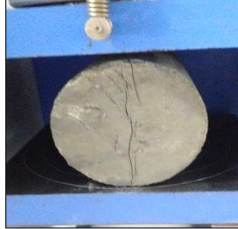
Fig. 5. Split tensile strength test
