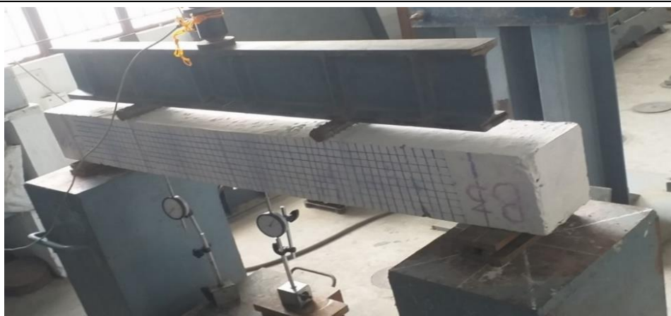
Fig. 9. Experimental setup of RC beam
