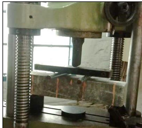
Fig. 6. Flexural strength test
