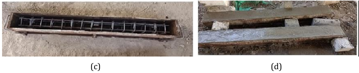
Fig. 7. Fabrication of the RC beams (a) Cross-section and longitudinal reinforcement details, (b) Steel mould, (c) Steel mould with reinforcement cage, and (d) Casting RC beams
