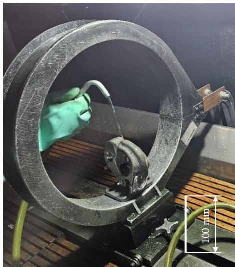
Fig. 2. Aircraft tow hook sample washing with magnetic particle testing solution
