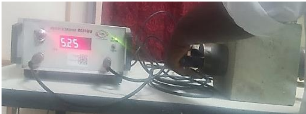
Fig. 9. UPV test set-up
