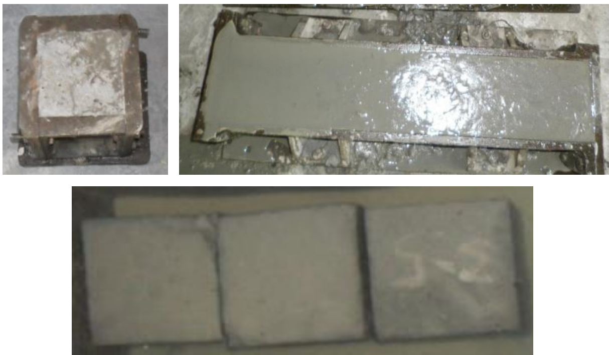
Fig. 6. Concrete poured into the mould and allowed to cure
