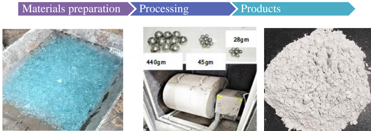
Fig. 2. Preparation of cementitious powder from WG
