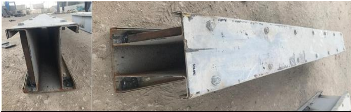
Fig 13. Failure Mode of Beam BH0.7
