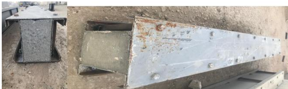
Fig. 20. Failure mode of beam BC1.3
