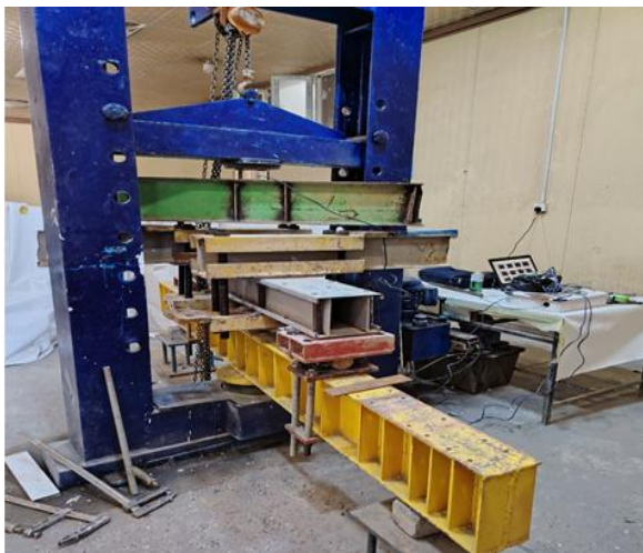
Fig. 6. Member under Torsional load
