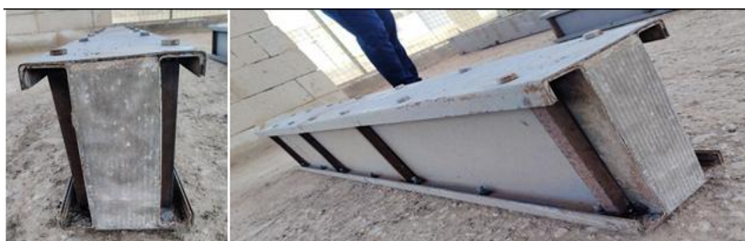
Fig. 24. Failure mode of beam BC0.7
