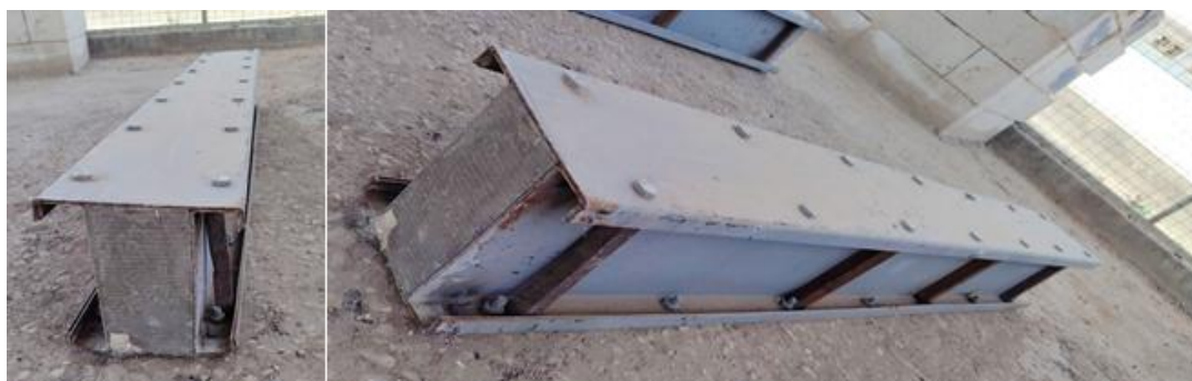
Fig. 23. Failure mode of beam BC0.85
