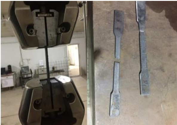
Fig. 4. Tensile testing machine with mounted specimen and tested coupons.
