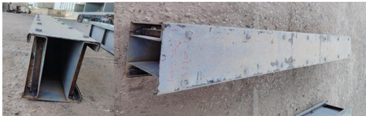
Fig 12. Failure Mode of Beam BH0.85
