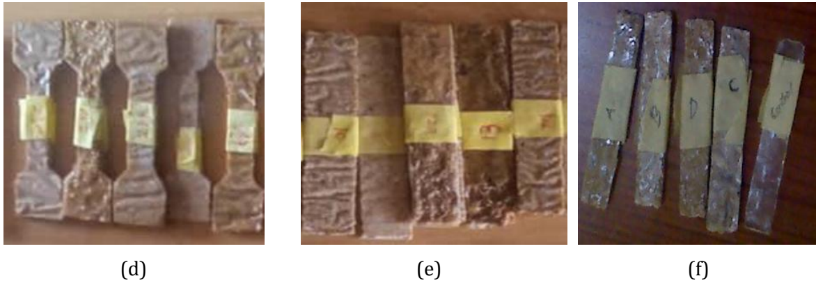
Fig. 3. (a) tensile mould, (b) flexural mould, (c) impact mould, (d) cured tensile samples, (e) cured flexural sample, and (f) cured impact samples
