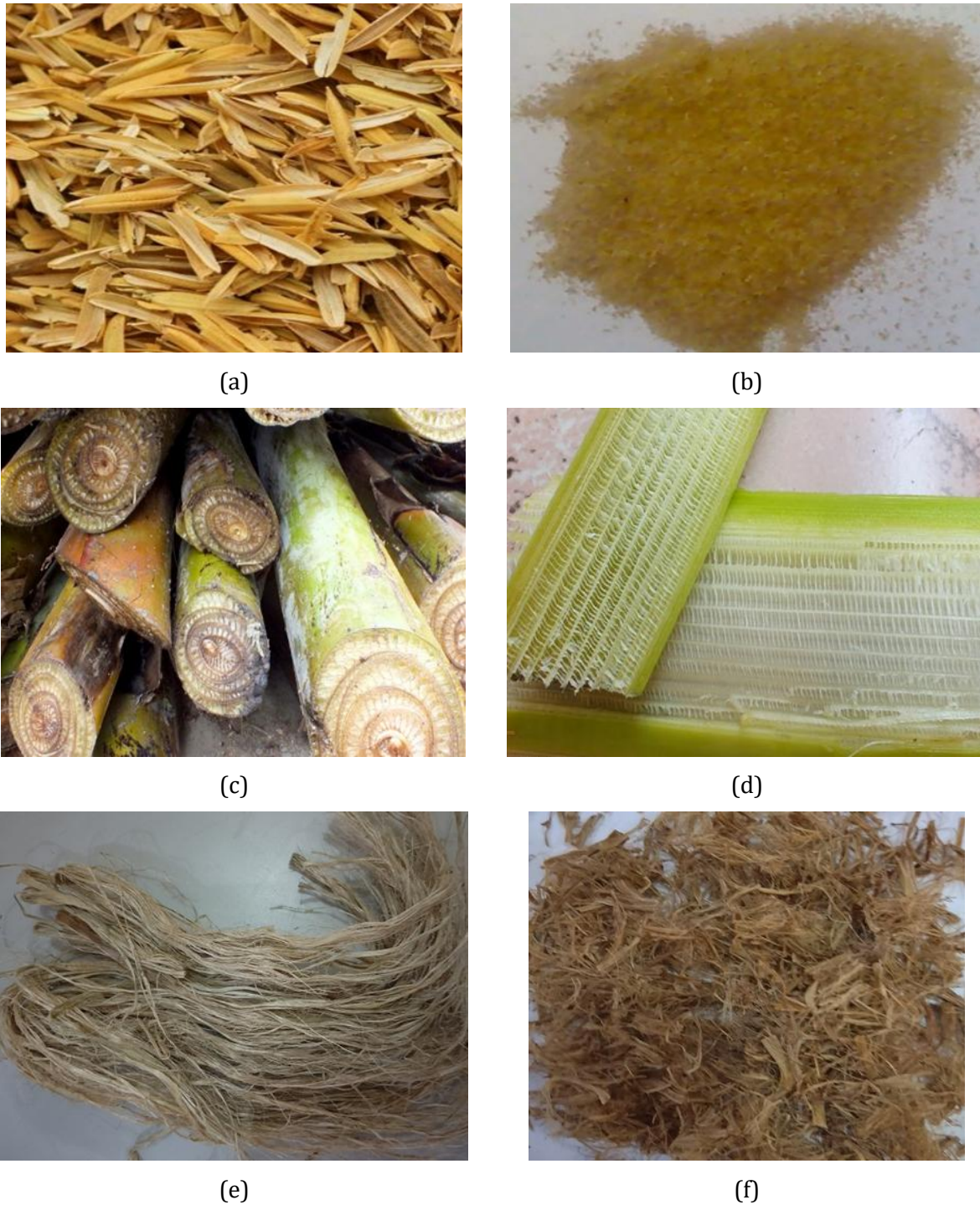
Fig.1. (a) rice husk, (b) milled treated rice husk (c) banana stem, (d) stripped banana stem, (e) extracted BF, and (f) chopped treated BF
