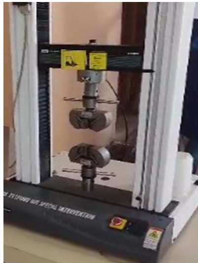
Fig. 4. Universal testing machine (Instron-3369)
